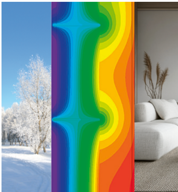
Image 1 Pronounced thermal bridge on aluminium consoles
