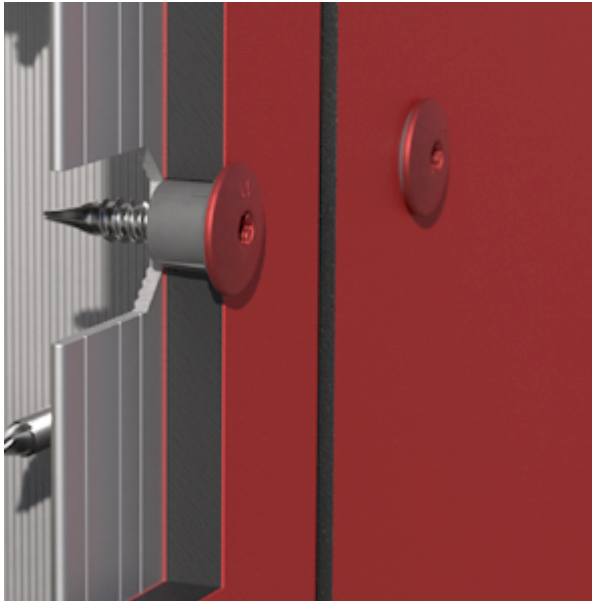
Detail view of fixed point for LT System
